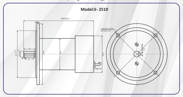
NOTE: 67MM LENGTH INCREASE FOR 200VDC @1000 RPM UNTOLERATED DIMNS. SHOWN ARE APPROXIMATE ONLY, ALL DIMENSIONS ARE IN MM.
